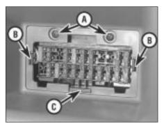
3.1a Method of fuse/relay board retention
